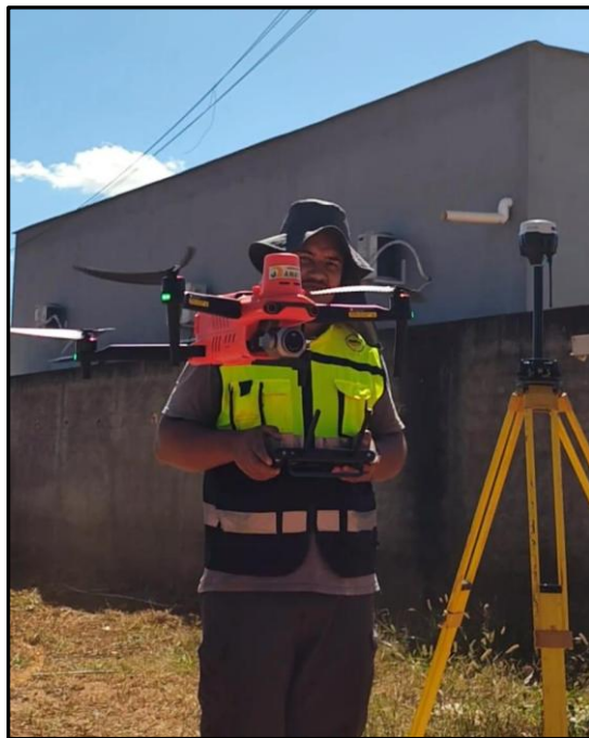
Figura 10: Drone EVO II Pro RTK V3 e o GNSS Emlid Reach RS2+.
