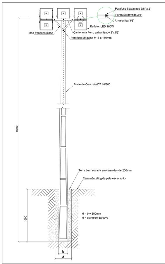
02 DETALHE - POSTE COM REFLETORES S/ESCALA
